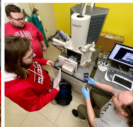
**Figure 4.** Loading sample M17-K808D01 into the Zeiss Supra SEM at CAMI for micro-textural and chemical analyses.
