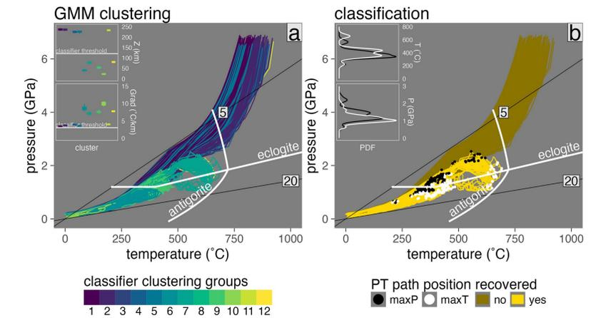
Example of marker classification. (a) Pressure-temperature (PT) diagram showing marker clusters as assigned by Gaussian mixture modeling (GMM; colored PT paths). (b) PT diagram showing marker classification results (colored PT paths) and various marker positions along their PT paths (black, white, and pink points).
